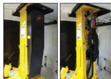
Emergency lowering valves located in pedestal within load area are safe and easy to access
