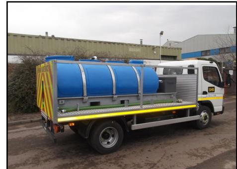
**Body Type and Specification:** 13 ft Long and 7 ft 6 Wide body. 18mm non slip alloy chequer floor. Alloy plank headboard and frame to rear end with chevron board. Fall arrest with detachable handrail. 3 point access. Pull out ladder to n/s
